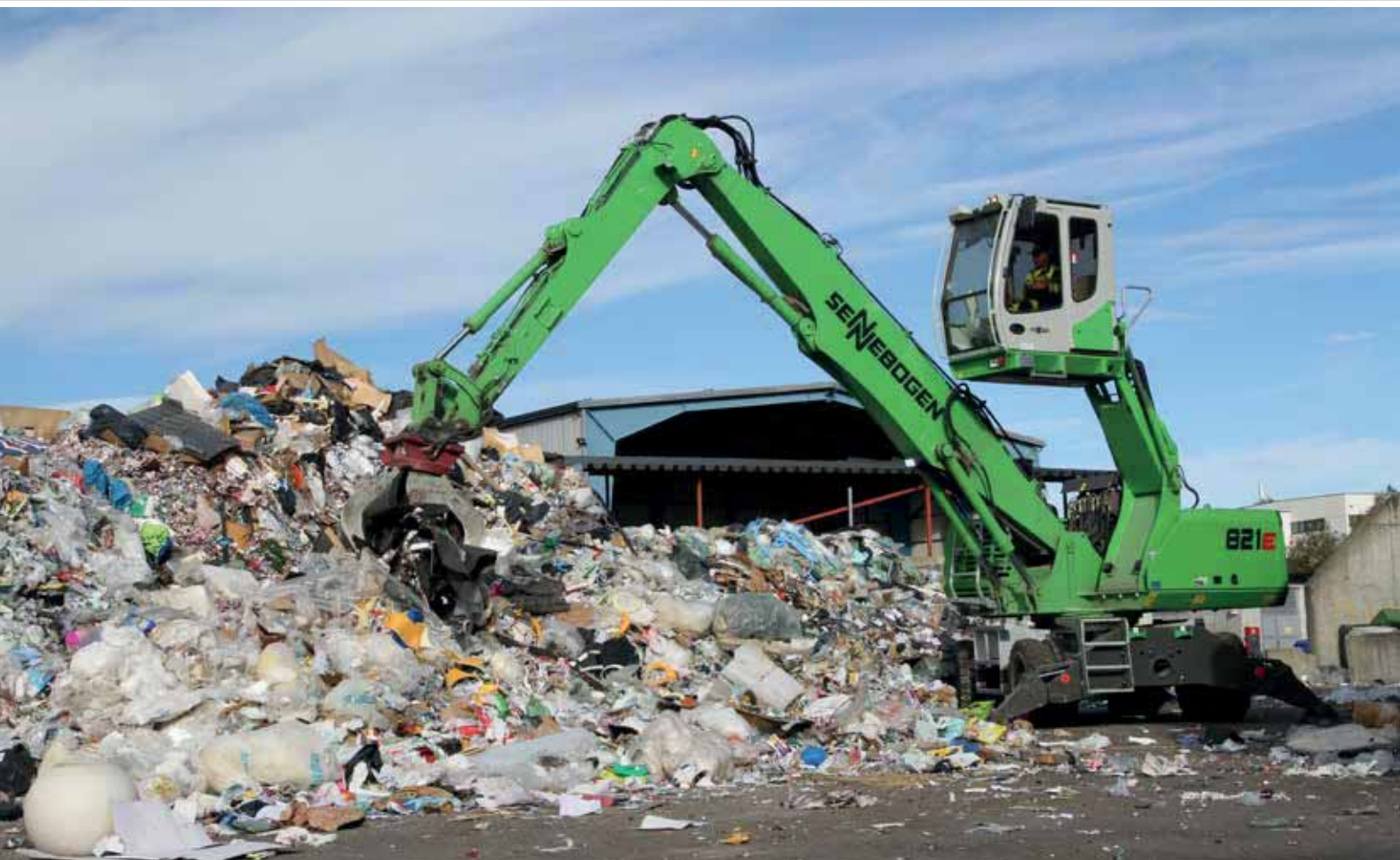
821 M – with orange peel grab – sorting waste; Norway
