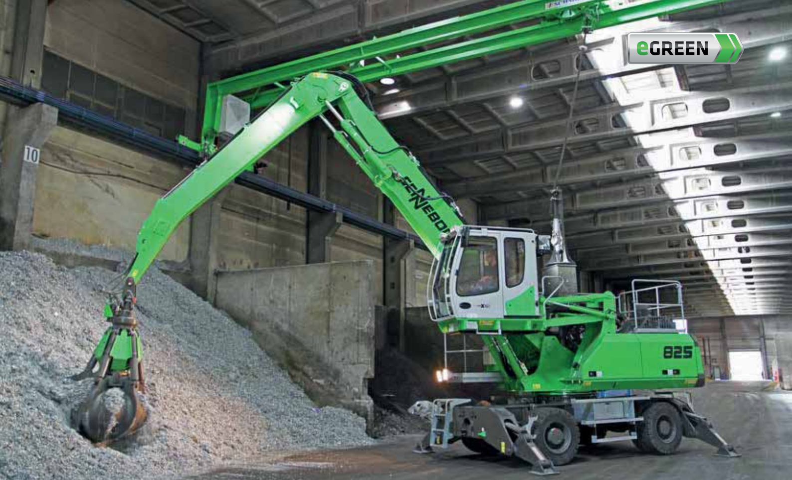
825 M Electro – with orange peel grab – scrap recycling indoor with ceiling power supply; Germany
