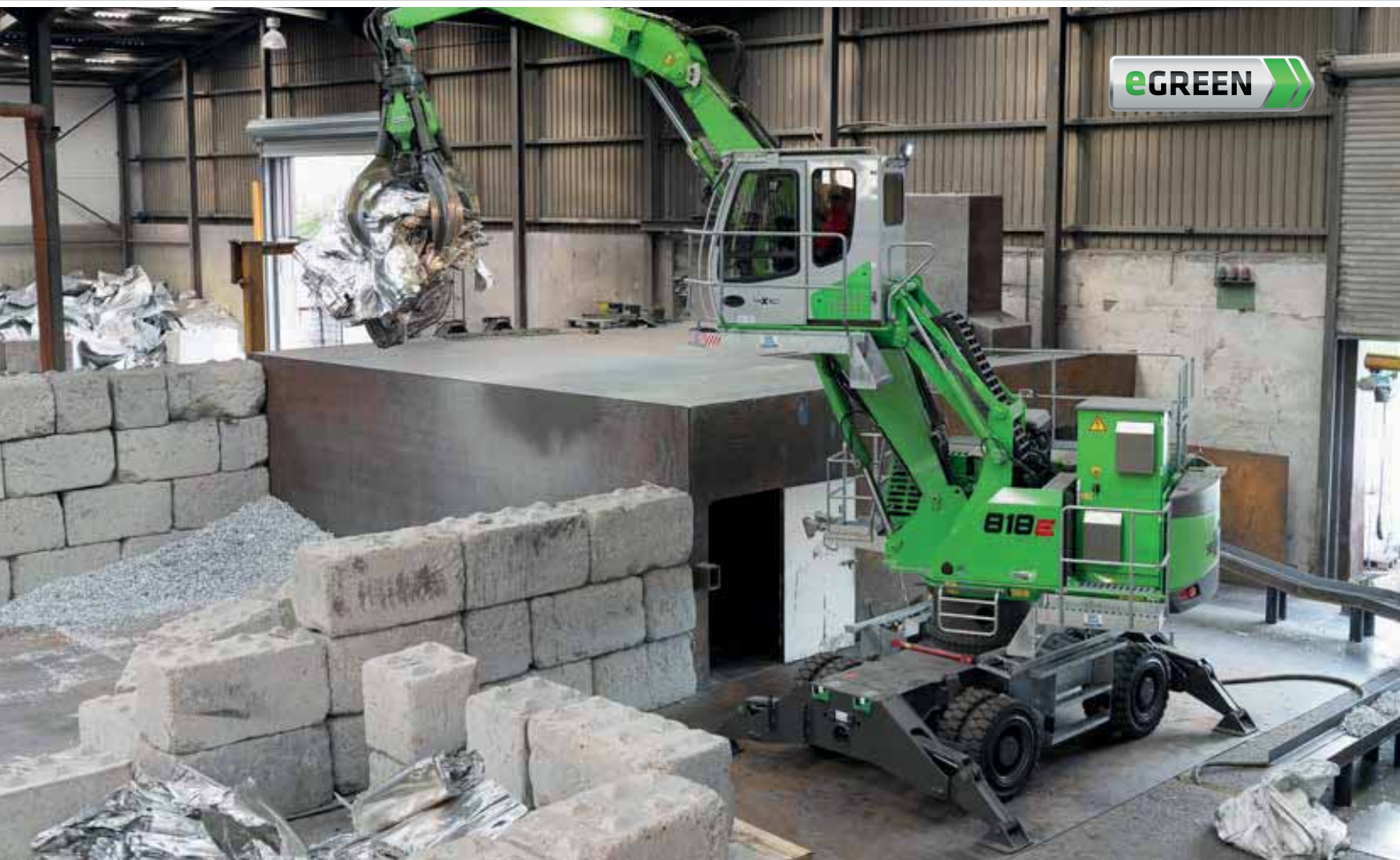
818 M Electro – with original SENNEBOGEN sorting grab – feeding of a baling press; Germany
