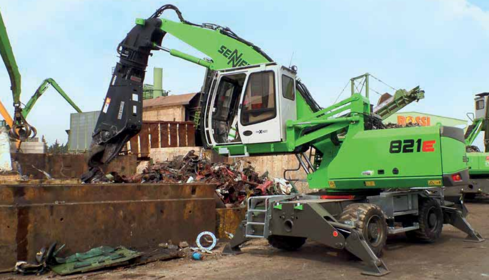
821 M – with 4 t scrap shear – shredding of scrap; France
