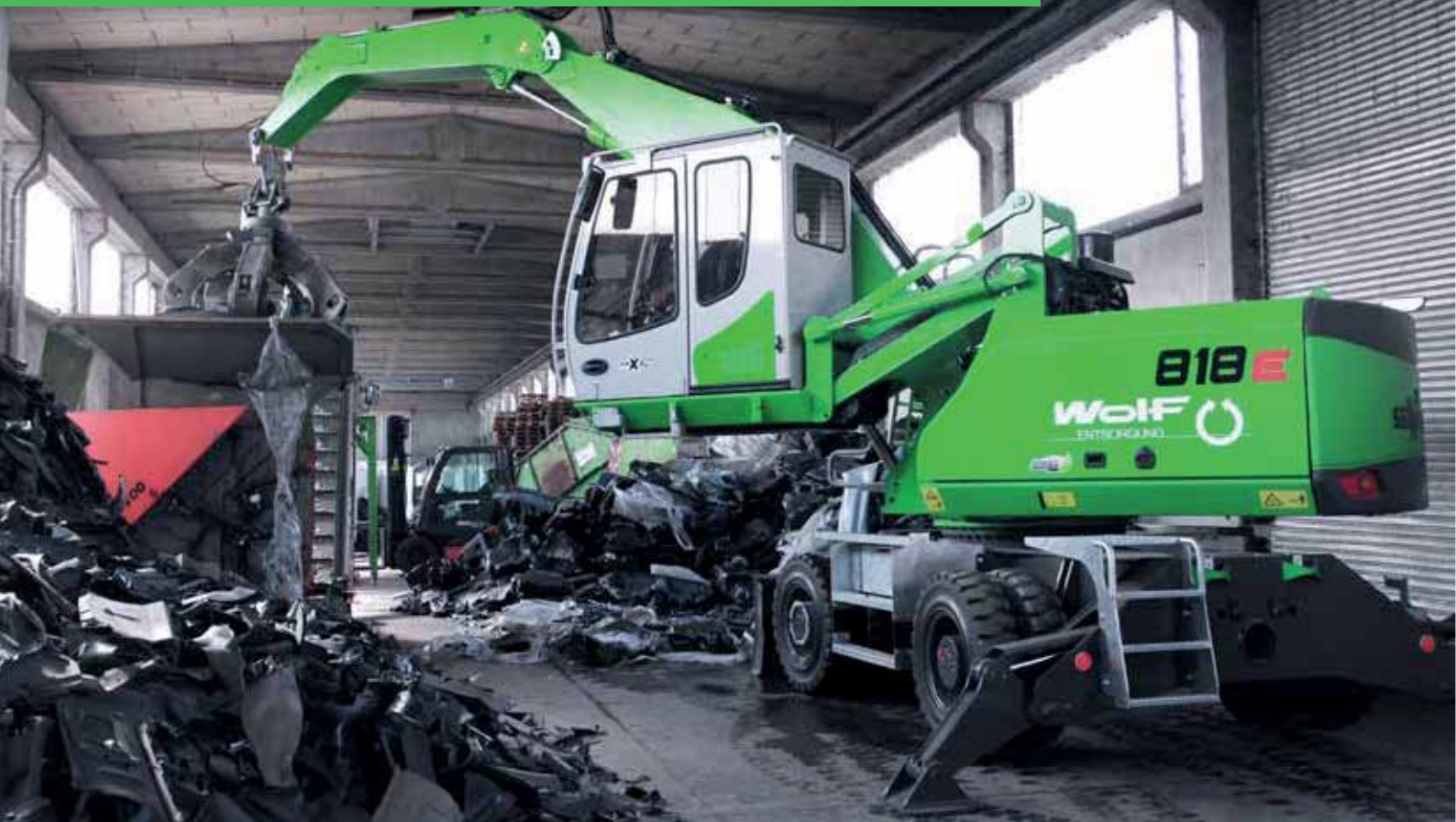
818 M – with orange peel grab – feeding a shredder with plastic inside a hall with low head room; Germany
