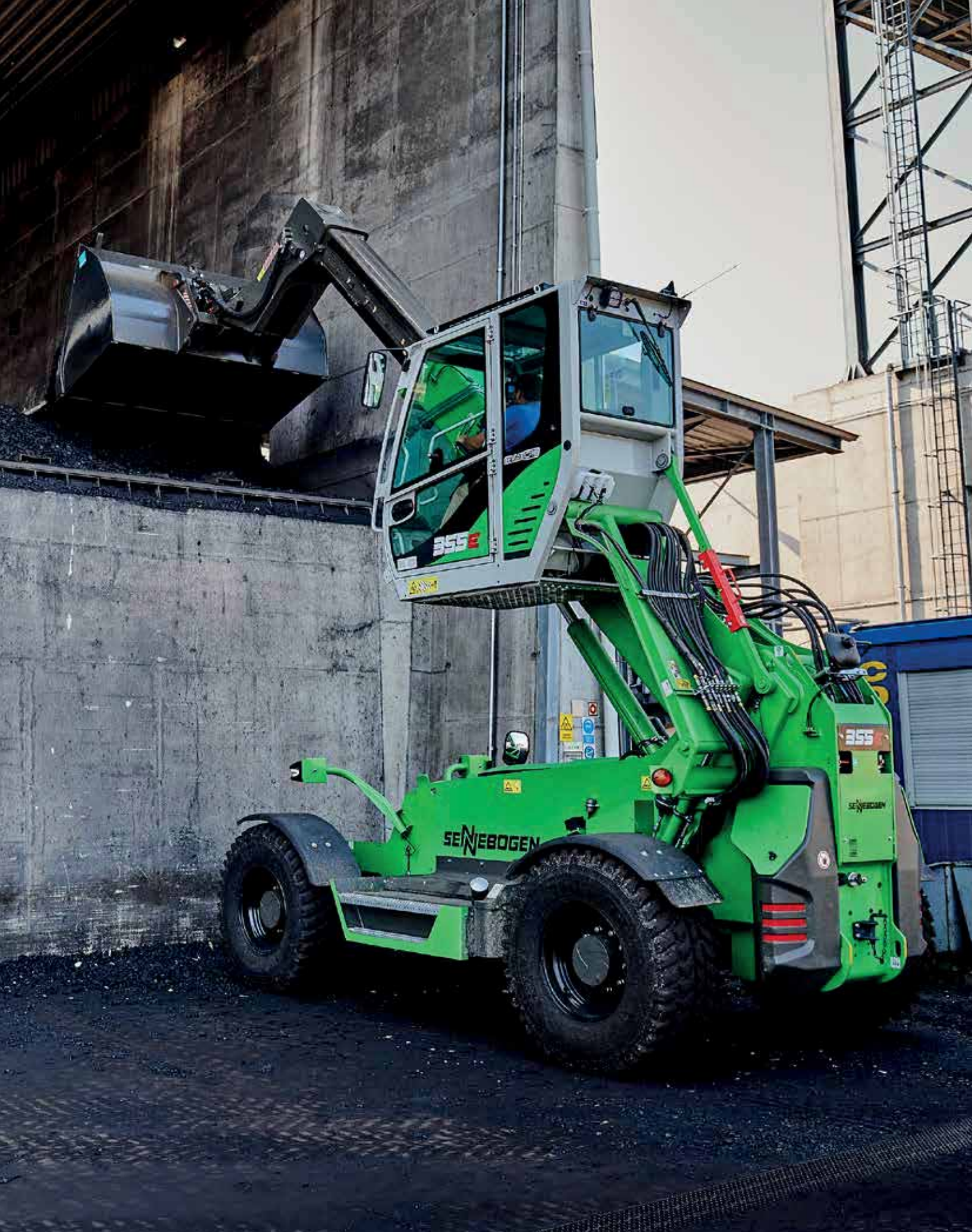
355 E Telehandler – powerful engine under dusty conditions thanks to standard reversible fan; Hungary
